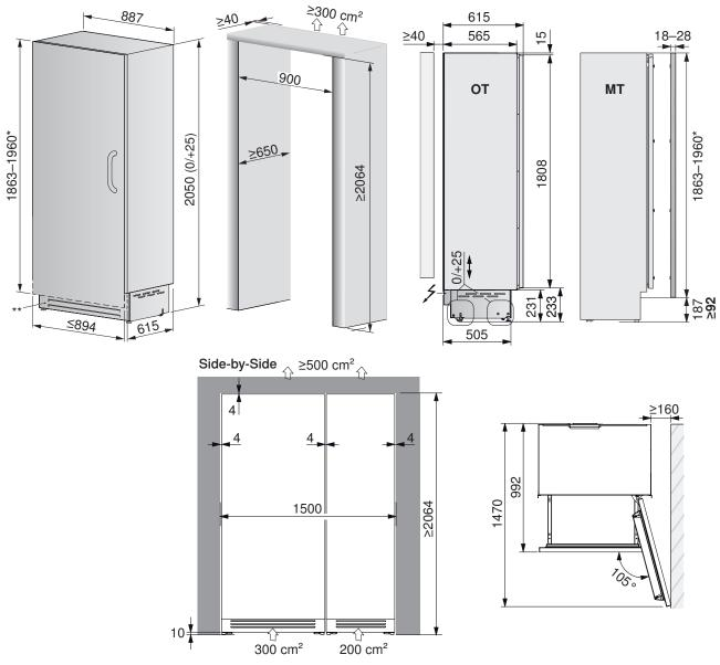
\* = For niche height >2064, drill holes in and height of door panel must be adjusted.
