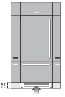
Dimensions for the ventilation grille and position of the magnetic strips
