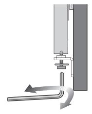
3) Align the door panel with the adjacent cabinets using the brackets and mounting brackets. By tightening or loosening the screw in the bracket, move the door panel up or down or, if the screws are loosened slightly, to the right or left to align it centrally with the rest of the kitchen cabinets.
