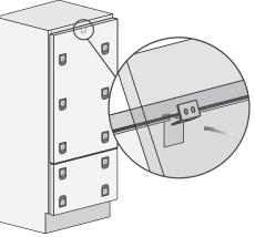
5) Hook the door panel into the mounting devices, starting from the top aligning brackets.
