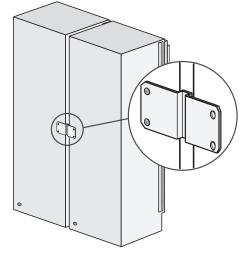
2) Fasten the mounting brackets on the back of the appli-► ances to connect them together. Fasten one side of the upper and the lower mounting brackets, first to one of the two appliances and then to the other.
