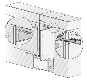
2) Fasten the appliance to the adjacent cabinets by screwing the lateral plastic connecting bracket onto the cabinets. This is easier to do if the door and drawer are left open.
