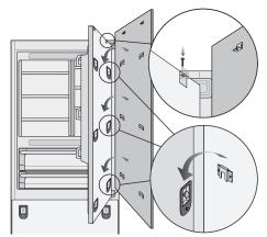
6) The door panel can now be adjusted to align with the adjacent cabinets using the brackets and aligning brackets.
