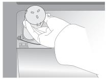
The filter is located behind the glass panel in the top of the refrigerator compartment.
