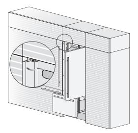
▶ 3) Push the cover strips sideways onto the brackets and then push in firmly until they engage with an audible "click".
