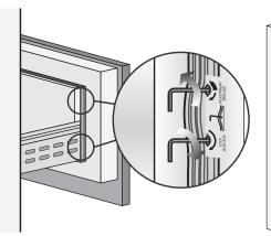
4) Depth alignment: From the inside of the drawer/door, lift up the seal. The top hole is for adjusting the door panel closer or further away and the bottom hole fixes the drawer/door.
