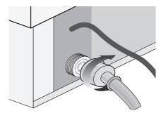
The scope of delivery includes an externally mounted water filter set. The water filter manifold and water connections must be prepared before the freezer is finally installed; the water connection at the back of the appliance to the water filter set must be in place before installing the appliance. Install the water filter set in a position where it can be easily accessed (such as in or below an adjacent cabinet) in order to be able to replace the water filter cartridge every 12 months.
