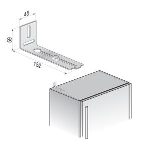
5) One or two brackets can be mounted around the intermediate area to act as an anti-tipping device or to prevent the appliances moving when the doors are closed. Brackets do not have to be screwed to the back wall.
